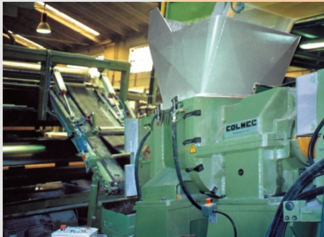
CTE 310 IN CONTINUOUS PRODUCTION AT 6.500 kg/h
